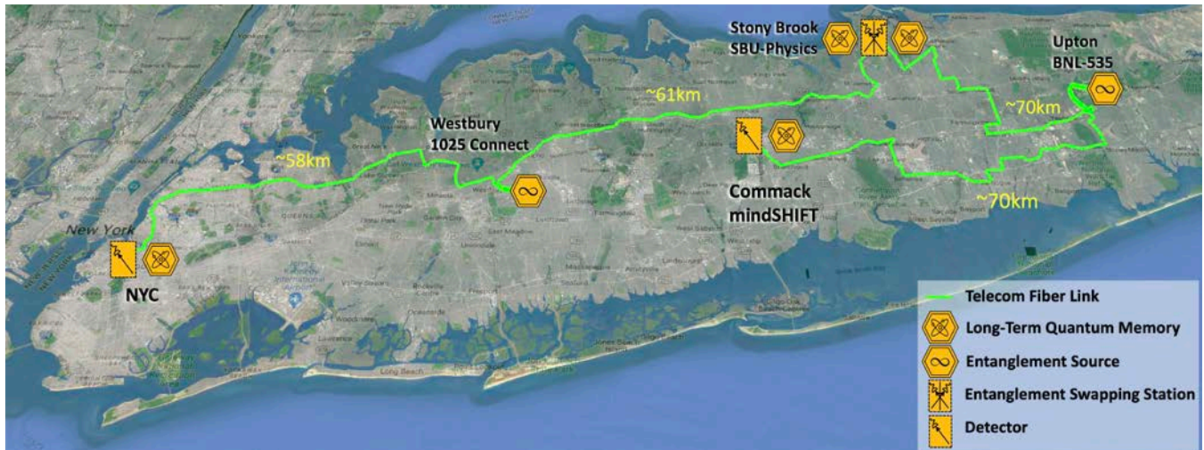
Figure 2: The Long Island Quantum Information Distribution Network (LIQuIDNet) testbed. Three Quantum nodes are located at BNL, SBU and NYC. They are connected using auxiliary nodes with entangled sources (1025 Connect colocation facility in Westbury) and heralded quantum memories (mindSHIFT in Commack). There exist two embedded physical optical networks: i) the quantum layer, that includes all quantum devices and forwards quantum signals and ii) the classical layer, for all other data signals, including timing and control. A separate digital control plane orchestrates the remote control of all quantum and classical devices in the network nodes. Figure courtesy Dimitrios Katramatos
